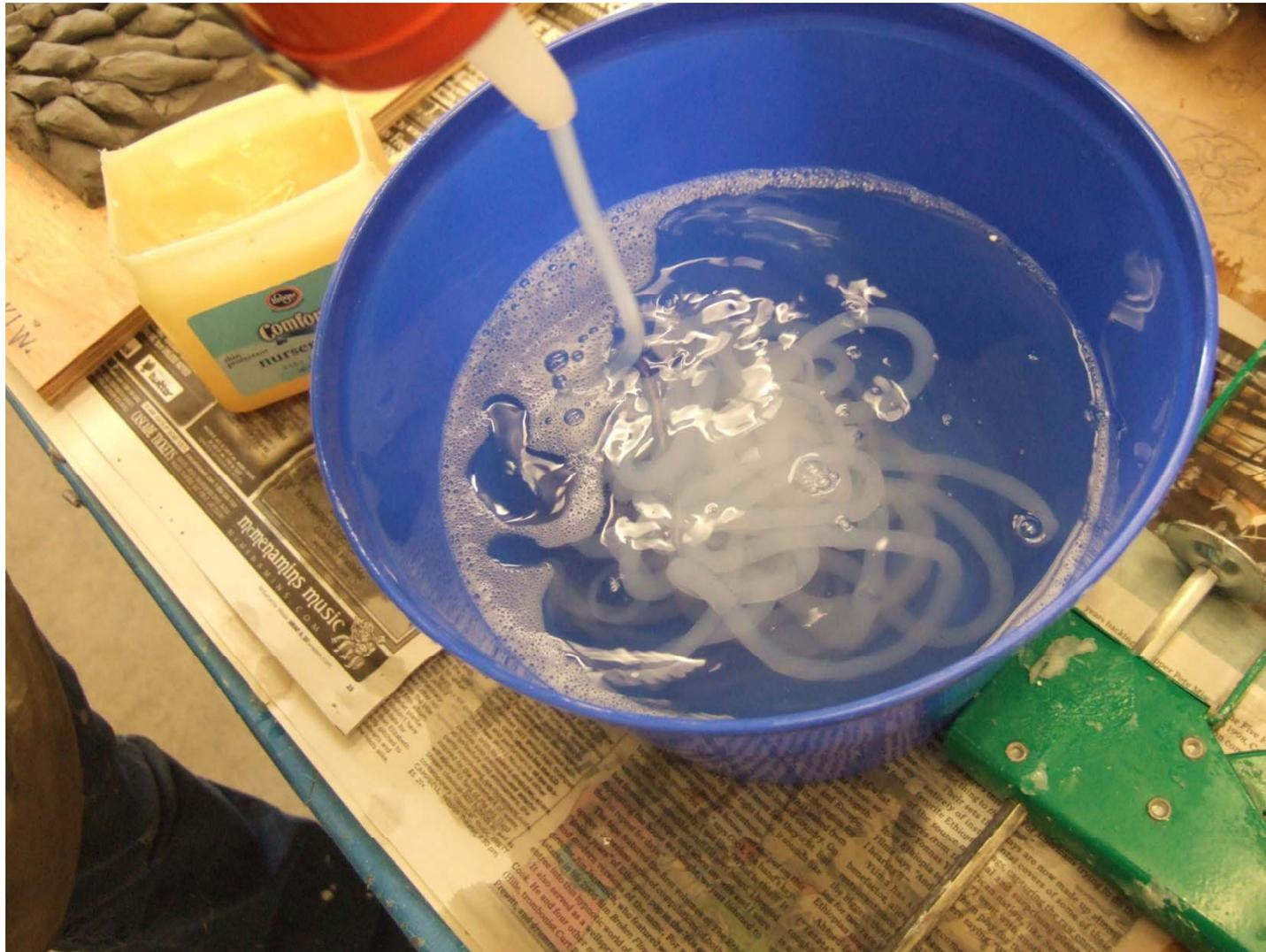
4. Depress the plunger of the caulk gun and empty the entire tube of silicone into the soapy water. (It doesn't have to be the whole tube at once if you're more comfortable with a few smaller amounts)
